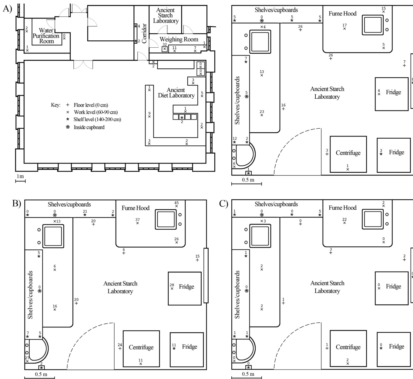
Fig. 1. Plan of RLAHA and the Ancient Starch Laboratory (ASL), Oxford, showing results of horizontal passive slide traps on A) work days, B) non-work days (ASL only), and C) after cleaning (ASL only); key in A) applies to all.
